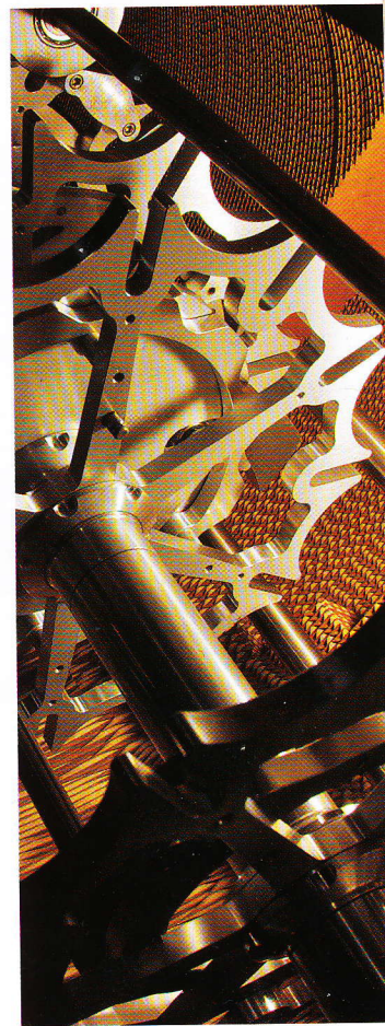
A detail of the clock's giant Geneva wheels.
